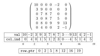
Fig. 1. An example of the three arrays (val, col\_ind, row\_ptr) used to store a matrix compressed sparse row (CSR) format.
